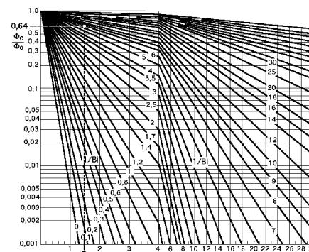
$$\text{por lo que: } Fo = \frac{t}{R^2} ; \quad 1,5 = \frac{0,0259 (\text{m}^2/\text{hora}) t}{0,025^2} \quad t = 0,0362 \text{ horas} = 2 \text{ min } 10 \text{ seg}$$
