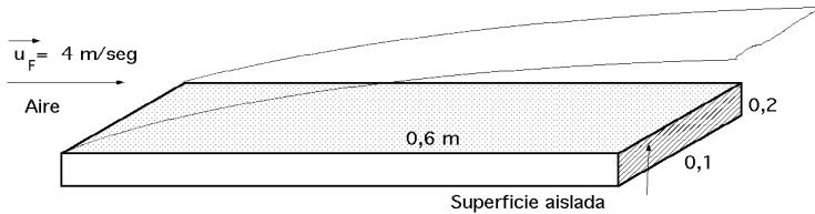
$$Re_L = \frac{u_F L}{F} = \frac{30 (\text{m/seg}) \times 0,6 \text{ m}}{17,6 \cdot 10^{-6} (\text{m}^2/\text{seg})} = 1,0227 \cdot 10^6 \quad (\text{Turbulencia desarrollada})$$
